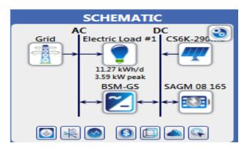
Figure 1. The schematic diagram of PV system model
